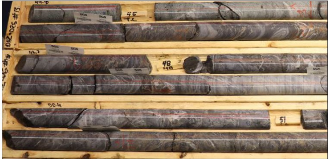
Figure 7-17: Dry core photo of Argillite from DHZ-026 at 48 m
