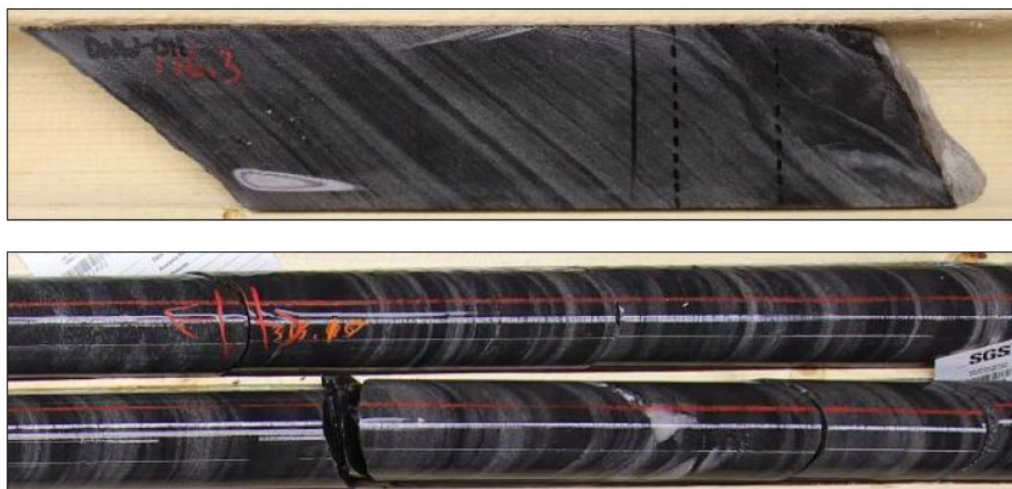
Figure 7-13: Wet core photo of Metasediments (3) from DNW-011 136.3 m and BR-060 315 m
