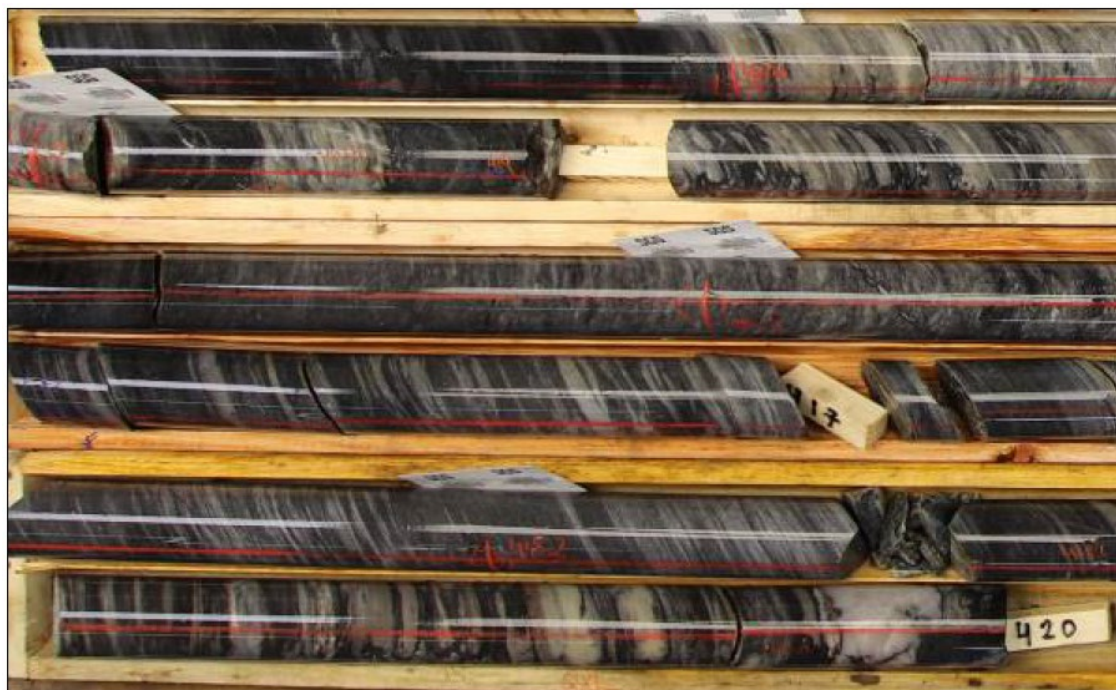
Figure 7-14: Wet core photo of Fragmental from BR-036 at 413 m to 420 m
