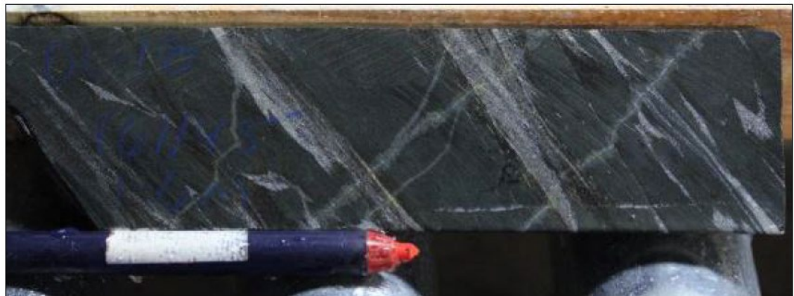
Figure 7-16: Wet core photo of Mafic Volcanic – Fe-Tholeiite – Biotite Calcite Pillows from DL-018 at 136 m
