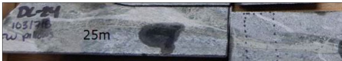
Figure 7-19: Dry core photo of Mafic Volcanic – High Fe-Tholeiite – Pillow Basalt from DL-024 at 25.0 m
