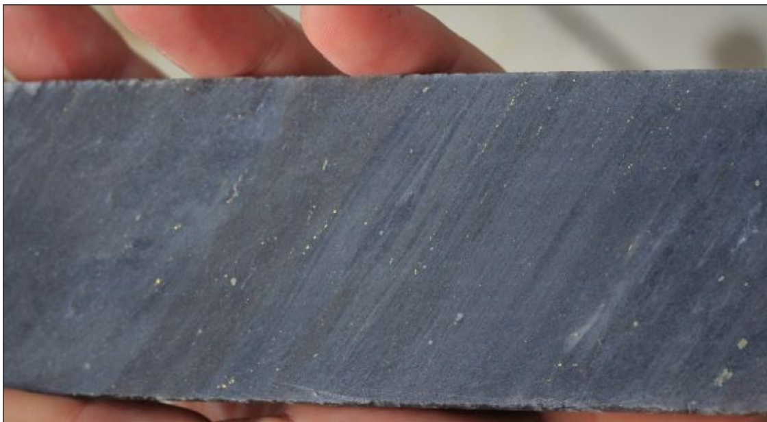
Figure 7-28: Strong strained Felsic Volcanic with 5% to 10% fine-grained arsenopyrite and 1% fine visible gold in the foliation in BR-020 at 90.15 m
