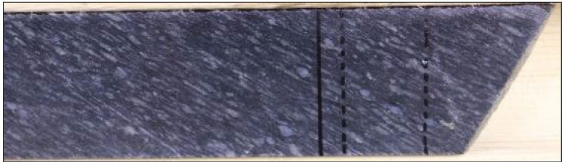
Figure 7-9: Wet core sample of Felsic Volcanic from DNW-011 at 13.2 m
