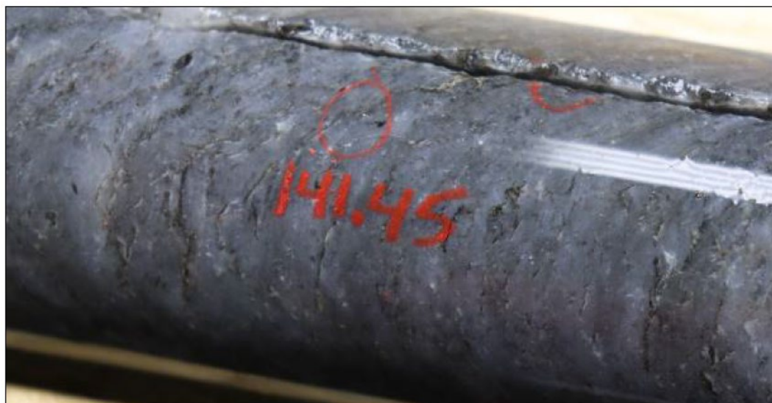
Figure 7-12: Wet core photo of Felsic Volcanic (2) from DNW-011 at 141.45 m
