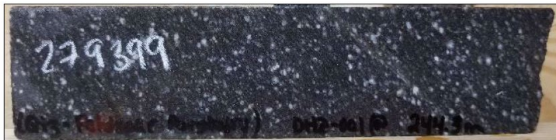
Figure 7-21: Wet core photo of Feldspar Porphyry Dyke from DHZ-001 at 244.3 m
