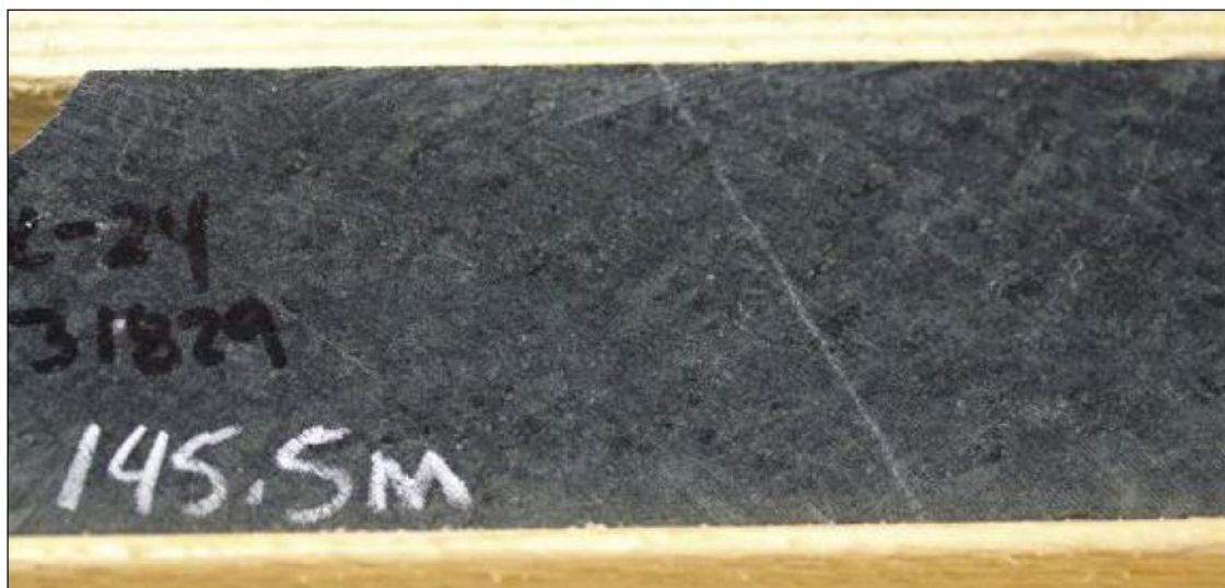
Figure 7-18: Wet core photo of Mafic Volcanic – High Mg-Tholeiite – Massive Basalt from DL-024 at 145.5 m
