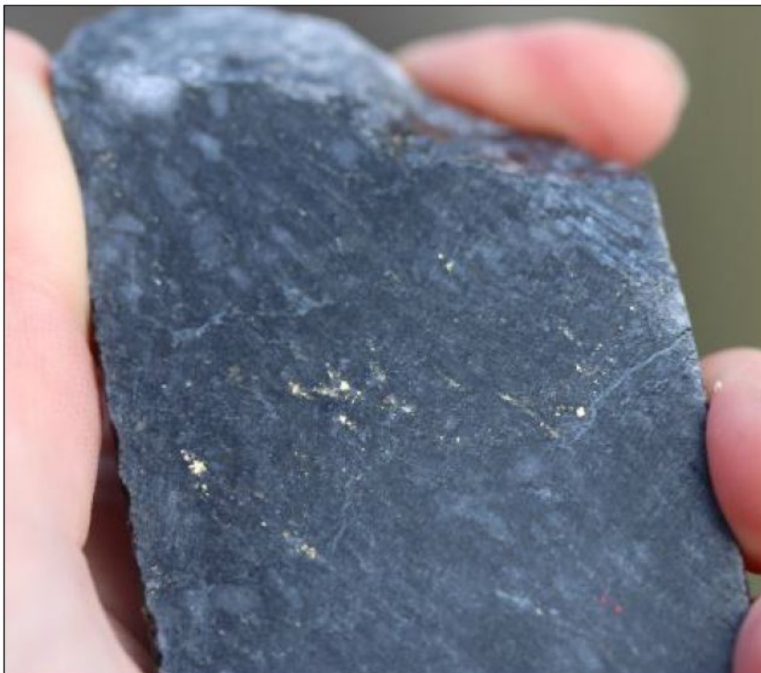
Figure 7-29: Visible gold in foliation hosted by strained porphyritic Felsic Volcanic from DNW-011 at 58.25 m
